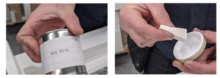
TIP: Using an angled makeup sponge as a brush to apply the paint will ensure a much smoother application due to the tiny pore size.
