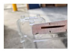
Apply exterior grade wood glue into both halves of the biscuit rebate and to one face of the end grain
