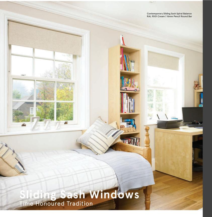
Bereco sliding sash windows have been designed to include traditional features whilst incorporating modern operation, technology and energy efficiency. Available in either spiral balance or cords and weights with an exclusive collection of decorative horns and elegant sash fittings.
